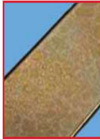
Typical silicate discolouration on the surface of the instrument after steam sterilization caused by excessive silicon dioxide levels in the demineralised water
