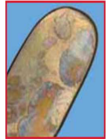
Typical silicate discolouration on the surface of the instrument after steam sterilization caused by excessive silicon dioxide levels in the demineralised water
