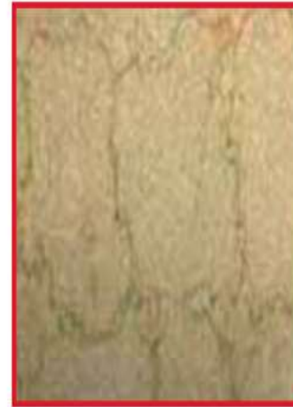
Typical silicate discolouration on the surface of the instrument after steam sterilization caused by excessive silicon dioxide levels in the demineralised water
