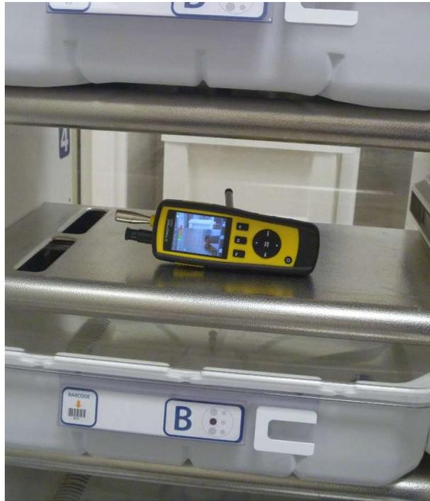
This sampling is undertaken removing all scopes and installing a particle meter in the geometric centre of the cabinet. This is an instrument that collects and analyses airborne contamination, similar in design to the active air sampler it draws air from inside the cabinet past a sensor that identifies the size and concentration of any airborne matter.
