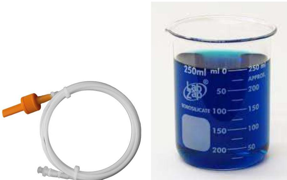
The surrogates are connected to all available relevant channel connections in the cabinet and the drying and storage program is instigated. With the distal end of the surrogate under 250ml of water the cabinet must have sufficient air flow and air pressure available to aerate each channel sufficiently. This same test is repeated for each position and channel connection option.
